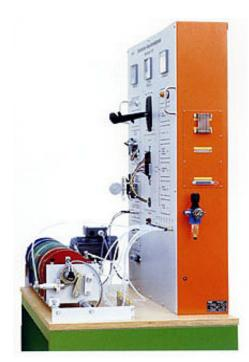
Measuring instruments for transmission input speed, transmission output speed, and vehicle speed are arranged clearly visible on the front panel.
